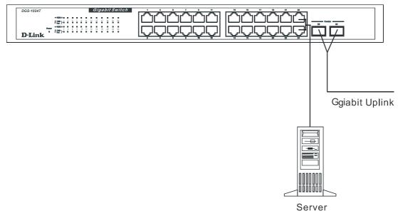
Figure 2- 6. Gigabit connection using optional module port
